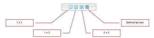
Large image display can present one or more images. How many images will be displayed, this can be selected by using these switches on the toolbar above the image display  $(1\times1, 1\times2, 2\times2)$ . Additionally the setting defined by user to maximum  $6\times6$  can be selected by using the last switch, which also opens the small window.
