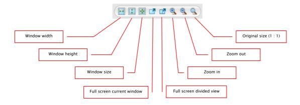
The options for zooming images refer in each case to currently active image. According to the standard the image display in a window is initialized in this way, that the image is scaled to the window size. If the size of the window changes in this option, e.g. by division of the image, the zoom factor is adapted accordingly, so that always the full image is seen.
